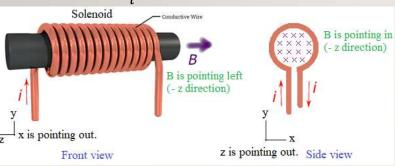
$\vec{\psi} = \vec{B} A$  where A is a cross-sectional area,  $A = \pi r^2$  where r is a radius of the coil.
